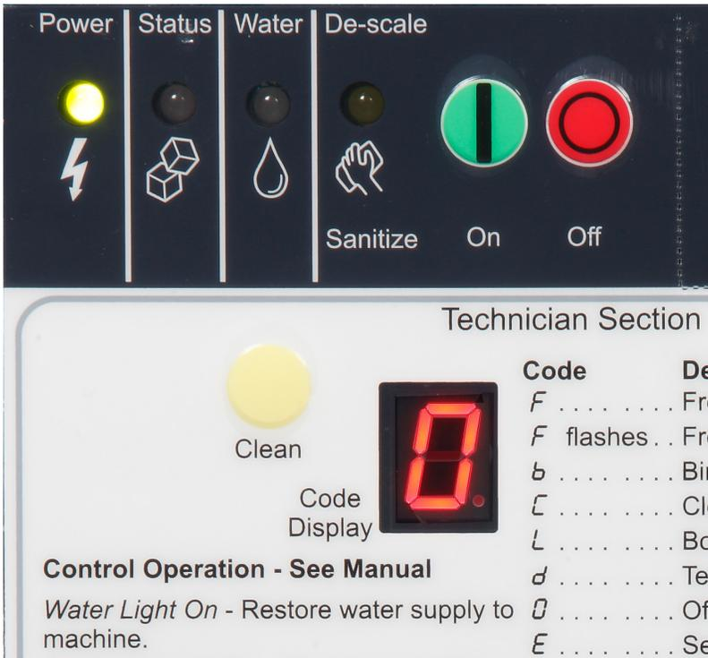
The control can be put into a Test Cycle, where it switches all the loads on and off in a logical sequence. This allows the technician to confirm controller operation of all parts.
