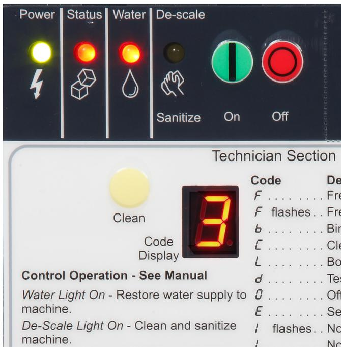
From the standby state, press and hold off button in for 3 seconds, then release it.
